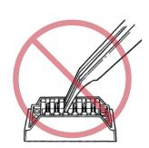
Applier jaws need to be positioned perpendicular to the cartridge body for slide-in of the jaw into the cartridge seat. It is necessary to set the shanks of the applier (the main body of the applier) at an acute angle to the cartridge.
