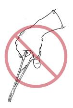
Grasping the applier at both rings tends to force applier tips together and "fights" the loading action. This may cause the applier to twist or rock, allowing jaw damage or misloaded clips.
